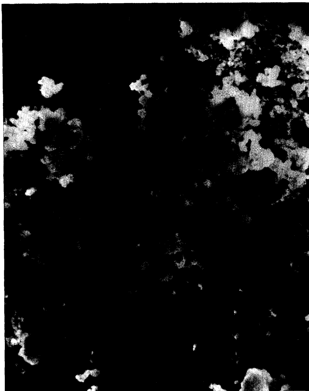
FIG. 2. Scanning electron microscope photograph of the surface of supported Ag catalyst containing a small amount of Ca, \gamma -irradiated and then heated at 300°C for 100 hr ( \times 4,402 ).
